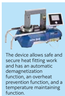
Fig. 15.42 Induction heater
